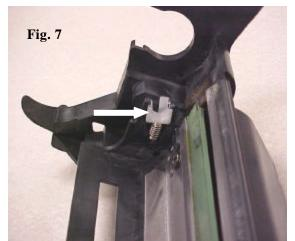
**10.** Remove both of the spring-loaded PCR saddles from the HP 2100 waste hopper.
