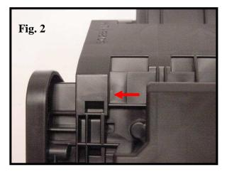
3. Once the hole is drilled in the correct area indicated in figure two the pin will be exposed (Fig.3). Do not remove the pin at this time.
