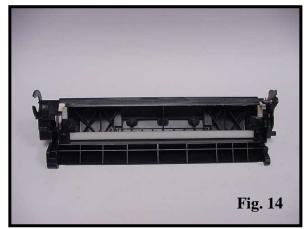
15. Clean or replace all components. Clean all contacts of conductive grease and re-apply. The drum stabilizer as well as the blue handle and tension spring are put back onto the cartridge once the two halves have been connected with cartridge pins. The remainder of the components in the waste bin can be reassembled at this time (Fig. 15).
