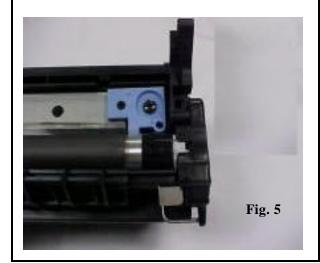
5. Once the contact end-cap has been re-installed, it should fit snuggly over the end of the toner low sensor bar.
