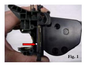
1. The toner hopper section must be completely disassembled, including removal of the Dr. Blade. Using a 1/8<sup>th</sup> inch drill bit, make a small hole as indicated in figure one.
